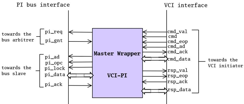
Fig. 3. Master Wrapper VCI and PI interfaces
