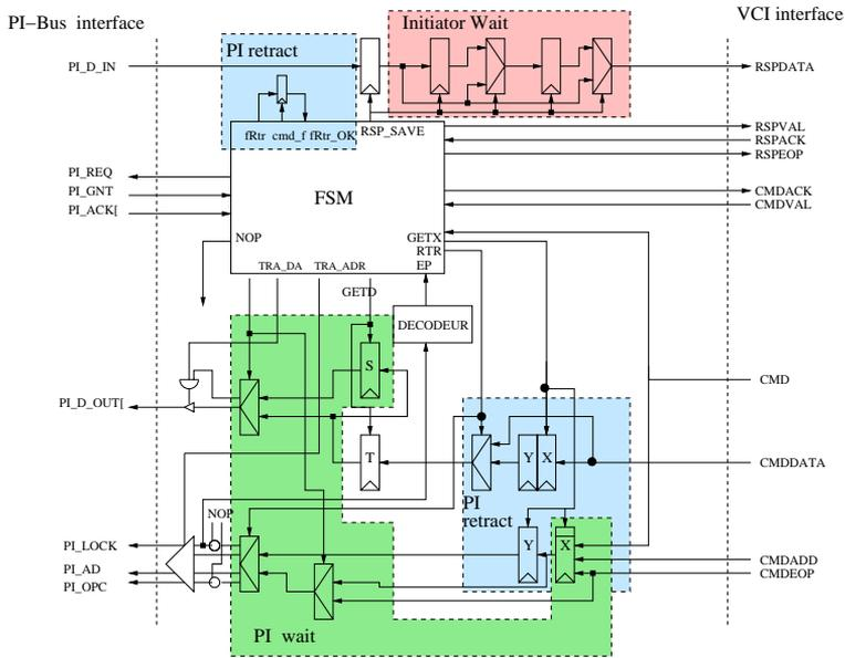
Fig. 6. Data-path of master wrapper C'. Each area corresponds to a different added increment.
