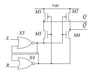
Fig. 6. Schematic of the arbiter.
