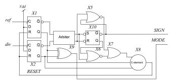
Fig. 5. Schematic of the bang-bang phase-frequency detector.
