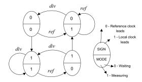
Fig. 4. State diagram of the bang-bang phase-frequency detector.
