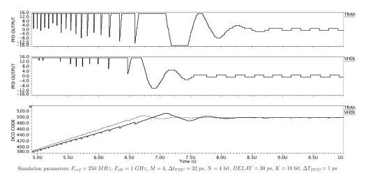
Fig. 8. The signed binary code (PFD output) and the control code of the DCO for fully VHDL code and transistor-level implementation.
