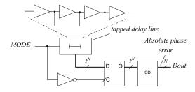
Fig. 7. Schematic of the time to digital converter.
