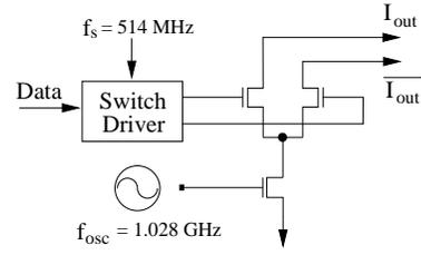
Fig. 5. Sinusoidal feedback DAC presented in [9], implemented in 1.8-V 0.18- $\mu$ m CMOS technology.
