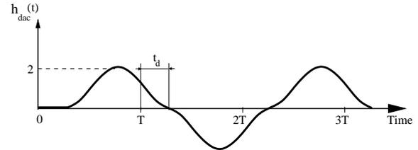
Fig. 2. Delayed sine-shaped feedback signal,  $h_{dac}(t) = 1 - \cos(\omega t)$ .
