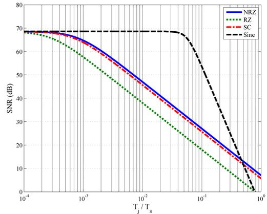
Fig. 2. SNR versus clock jitter of a 4th order bandpass CT ADC with OSR=64 for different types of feedback DACs [8].
