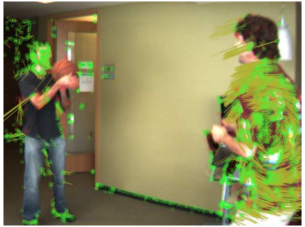
Fig. 2. Optical flow detected with L1P at Basketball sequence second frame. Displacement vectors in yellow are displayed magnified.
