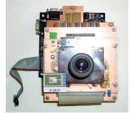
Fig. 6. PARIS1 based vision system
