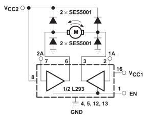
Figure 5. Bidirectional DC Motor Control
