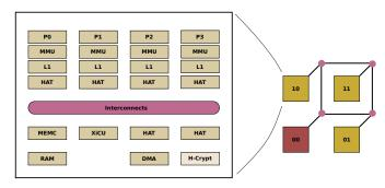
Figure 1. Example of standard cluster in TSAR architecture.
