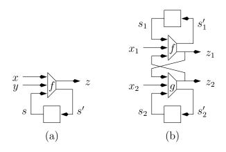
Figure 1: Synchronous machines and their composition
