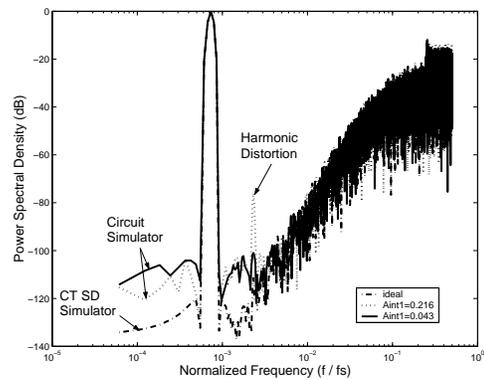
Fig. 10. Comparison between ideal system-level  $\Sigma\Delta$  simulation and circuit level simulation.
