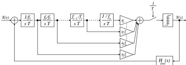
Fig. 5. Scaling factors are introduced to limit integrators output swing.
