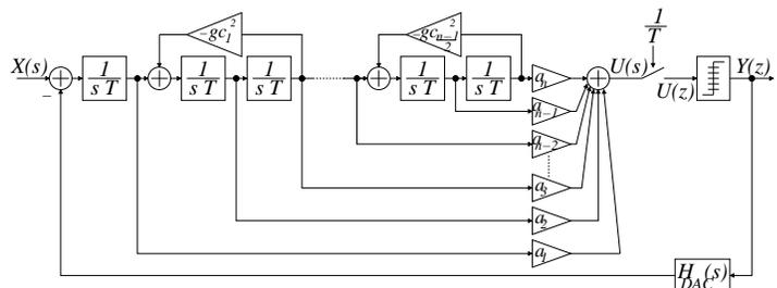
Fig. 2. General form of a continuous-time  $\Sigma\Delta$  modulator.
