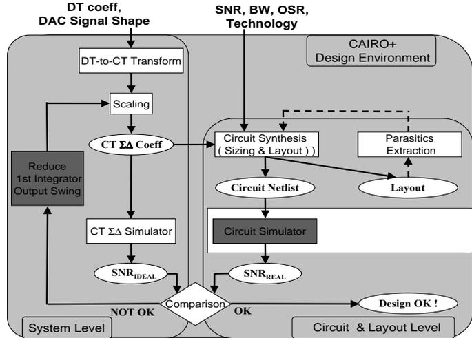
Fig. 1. CT  $\Sigma\Delta$  modulator synthesis in the CAIRO+ design environment.
