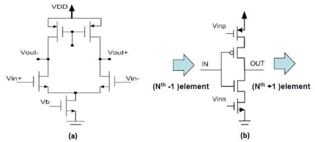
Fig. 9. (a) Single stage opamp circuit (b) Ring-VCO unit cell
