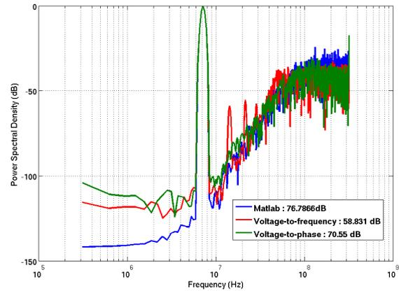
Fig. 10. Output power spectral density of a transistor level simulation of a 4<sup>th</sup> order CT  $\Sigma\Delta$  modulator with voltage-to-frequency quantizer compared to voltage-to-phase quantizer with only the DACs ideally modeled.
