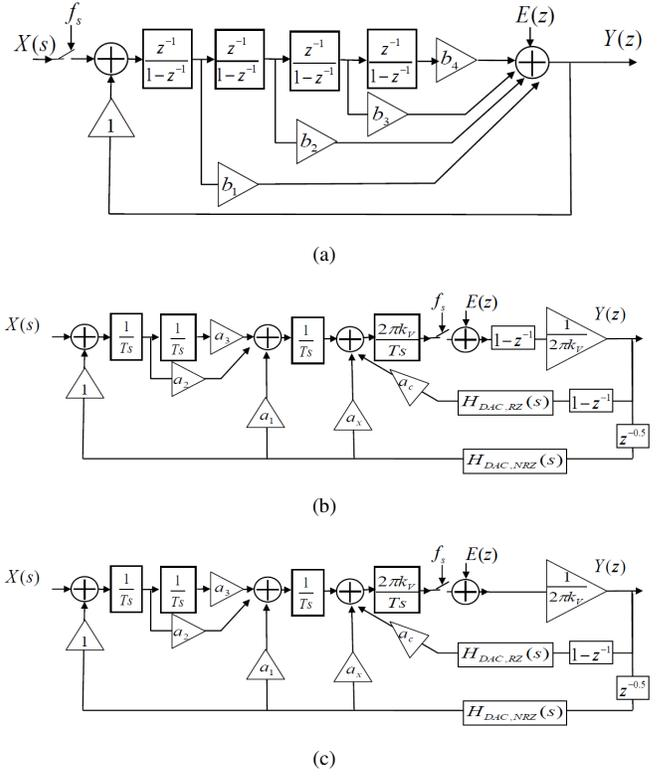
Fig. 6. 4<sup>th</sup> order  $\Sigma\Delta$  modulator CIFF (a) DT (b) CT with voltage-to-frequency quantizer (c) CT with voltage-to-phase quantizer
