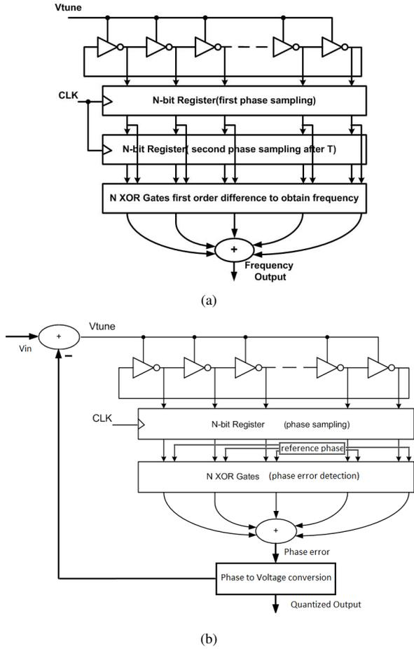
Fig. 3. VCO-based quantizer implementations (a) Voltage-to-frequency (b) Voltage-to-phase .
