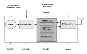
Fig. 2. Structure of a wireless sensor network mote.
